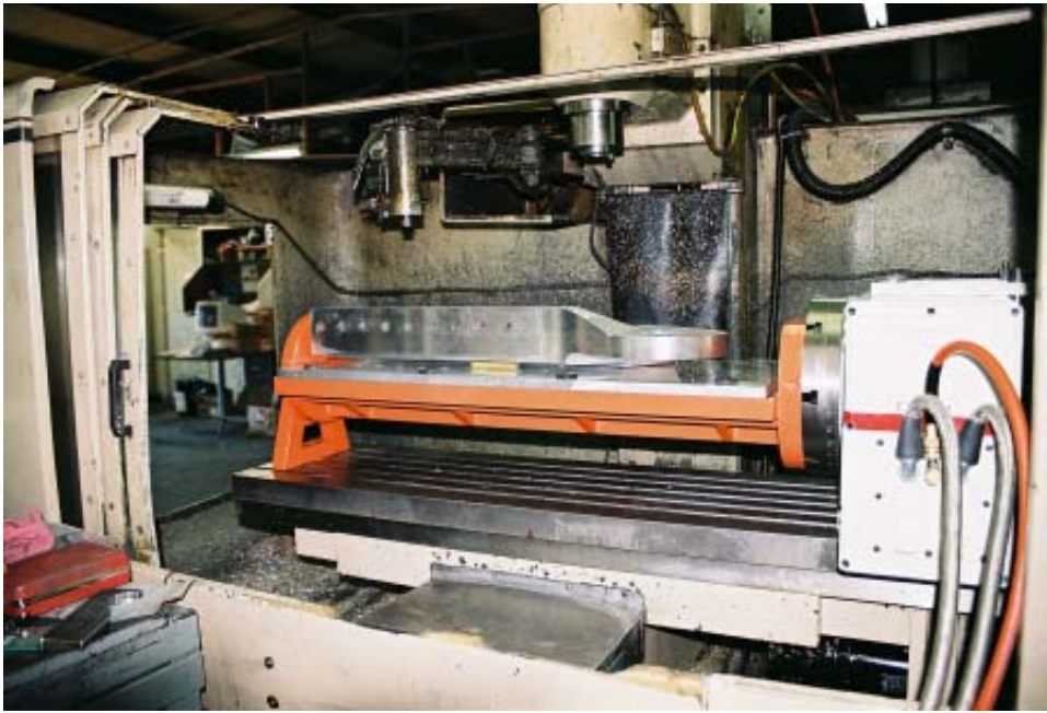
Military Part being machined on 3 sides using an SMW Indexer
